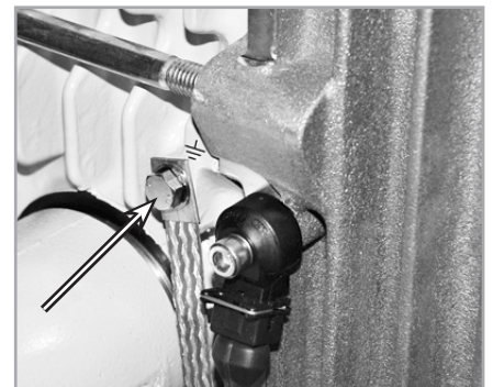
Fig. 3.6 Ground connection example
