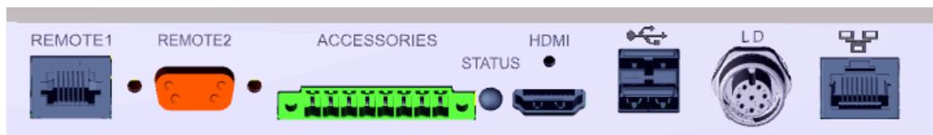
Fig. 6: Connections for accessories and control signals at the back side of the device.
