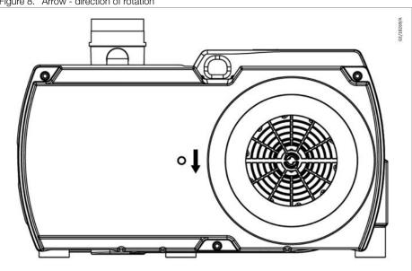
Figure 8. Arrow - direction of rotation
