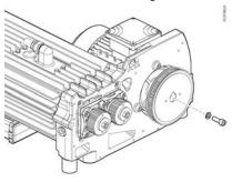
14. Remove the pulley with the gear puller tool and M8 hexagonal screw.
