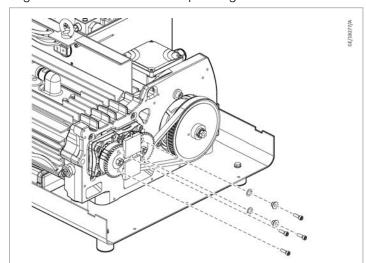
4. Tighten both the steel and the plastic gear with 2 bolts each to 10 Nm.
