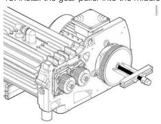
15. Unscrew the 4 motor screws. Hold the motor while unscrewing and unscrew the uppermost screw last.
