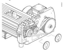
9. Install the gear adjustment tool on the fail safe gears.
