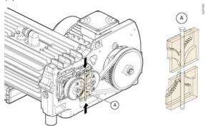
6. Loosen and remove the bolts of fail safe gears.
