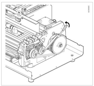
2. Push the motor towards the pump body to loosen the belt.
