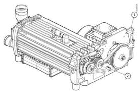
2. Install the 4 motor screws and hand tighten.
