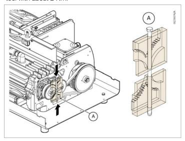
3. Loosen the 4 bolts fixing the gears with a 5 mm Allen key and remove the bolts.
