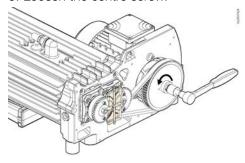
7. Remove the gear fixation tool.
