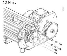
10. Assemble the fail safe gears bolts and tighten with
