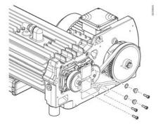
8. Remove the fail safe gears.
