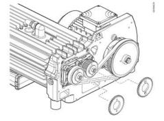
9. Loosen the 4 motor screws.
