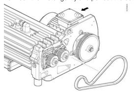
12. Install the M8 hexagonal screw.
