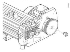
13. Install the gear puller into the middle of the pulley.
