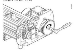
13. Tighten the motor screws by following steps 2-7 in Assemble tooth belt on page 33.
