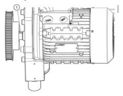
6. Insert the centre screw and hand tighten.
