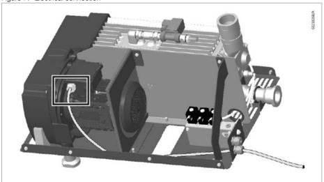
After connecting the motor and after every time you alter the wiring, check the direction of rotation. To do so, briefly switch on the motor and make sure
