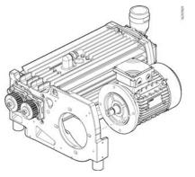
3. Install the pulley to the motor.
