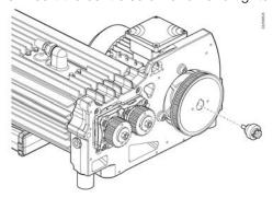
8. Assemble both fail-safe gears. Replace the plastic fail-safe gear if it is worn.
